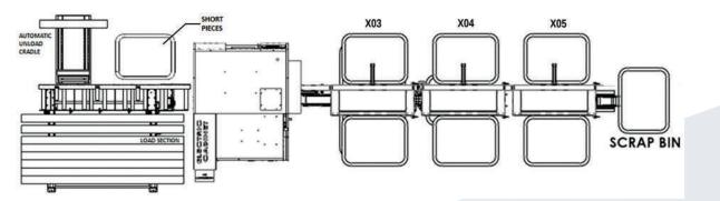
STANDARD AMSAW 70,125,180,250,350 COMPACT AUTOMATIC HIGH PERFORMANCE SAW SYSTEMS WITH AUTOMATIC LOAD AND UNLOAD UNITS FOR 12FT AND 20FT BARS WITH EXIT GRIPPER POWER CONVEYOR PART UNLOAD SYTSEM WITH 6 BIN STORAGE AND SCRAP BIN.
